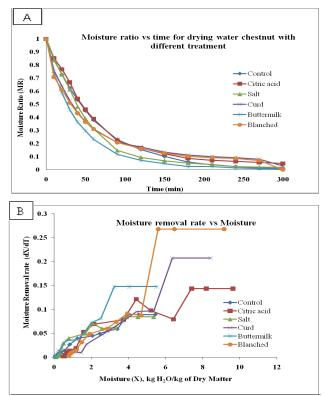
Figure 1. (A). Time vs. moisture ratio for drying of water chestnut with different treatment; (B). Moisture (X) vs. moisture removal rate (dX/dT)
